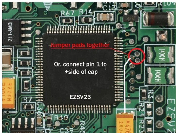
**EZSV17:** PCB Pre and including Rev J02, locate the two pads next to the processor (circled in red) and short them together with solder.
